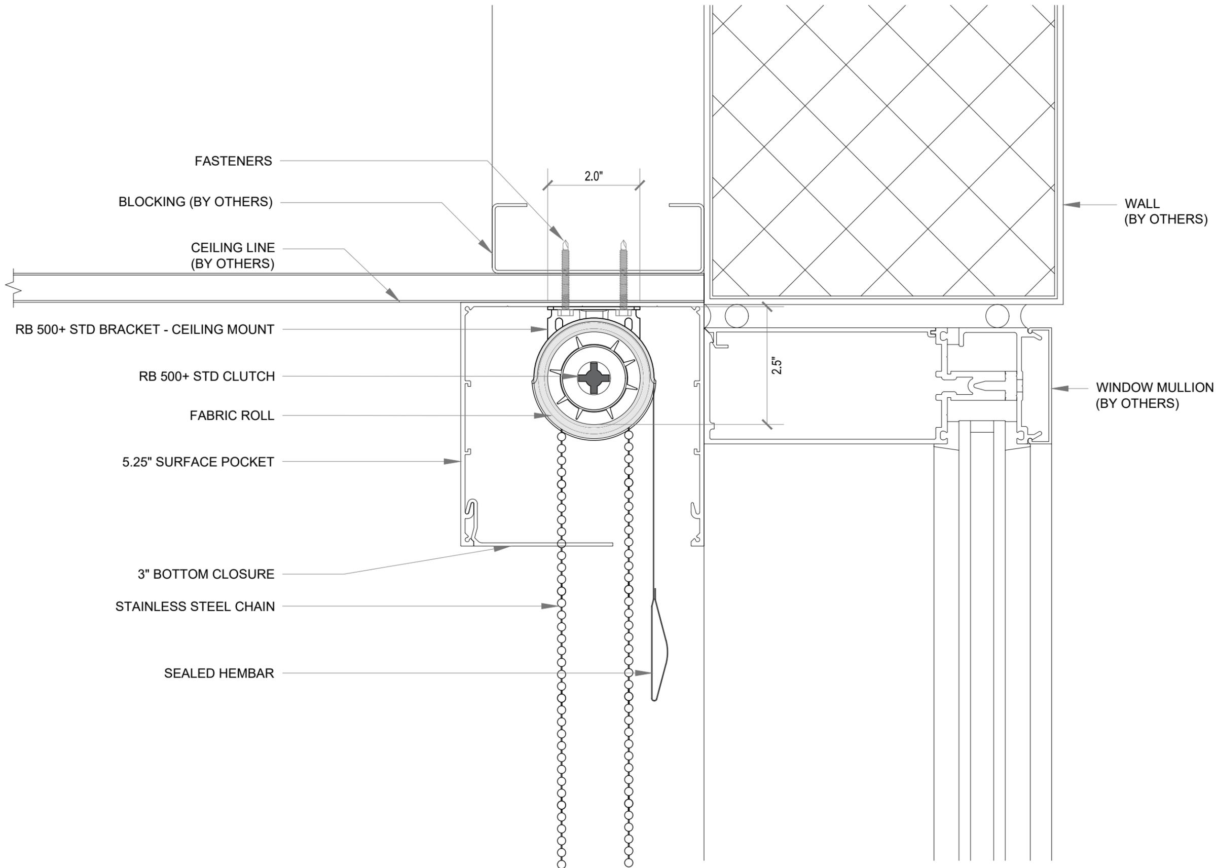
**01** RB 500+ STANDARD DUTY BRACKET 38 - SECTION DETAIL
